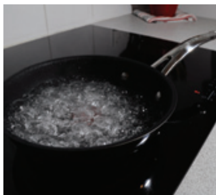
Induction cooktops have a flat, smooth cooking surface that isn't hot to touch when the power is turned on
